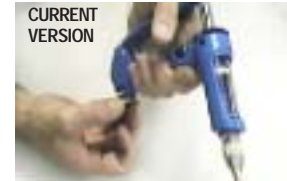
Loosen the needle nut and insert the needle, then re-tighten the needle nut.
